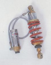
for compression, and 30 settings rebound damping, as well as adjustable spring preload. The rear shock offers 16 different positions for compression and 19 for rebound, as well as preload adjustment and a remote reservoir. Whatever your
