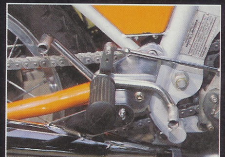
The rear brake is actuated by a "dual-action" heel-toe lever. Makes slowing down double the fun, especially at high speeds!
