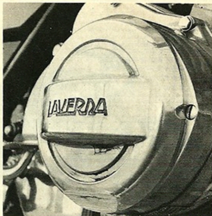
The alternator/ignition unit's cover suffers when right-hand turns are made at immoderate speeds.
