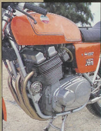
Above: The two outside pistons fire simultaneously.
